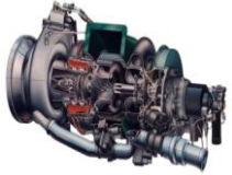
Auxiliary Power Unit
