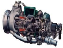
Auxiliary Power Unit
